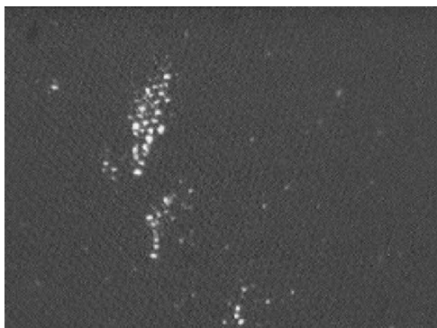
Fig. 18 Optical microscope image of clump of holes in A1 film described in face B2 feature 2.
